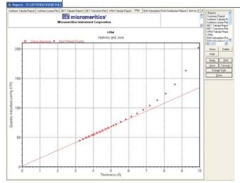
The Gemini VII 2390 Series analyzers provide rapid surface area analysis. The unique balanced design allows BET surface area to be measured using nitrogen for a broad range of materials. The Gemini offers precise measurements of low surface area materials using nitrogen. The determination of micropore volume, micropore surface area, and external surface area is available on all Gemini models using the standard t-plot calculations.
