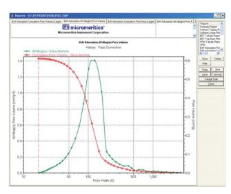
The Gemini VII 2390p includes a dedicated transducer for continuously monitoring the saturation pressure of the cryogenic bath. This allows the Gemini VII 2390p to rapidly measure adsorption isotherms and determine the pore volume, area, and size distribution of mesoporous materials.
