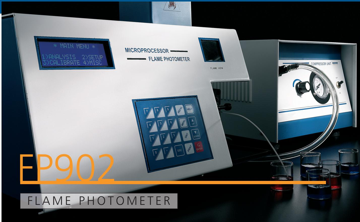
The PG Instruments FP902 Flame Photometer offers the combination of clinical, industrial and education applications in ONE instrument. It gives accurate, fast and precise analysis of sodium, potassium, calcium and lithium in one simple aspiration.
