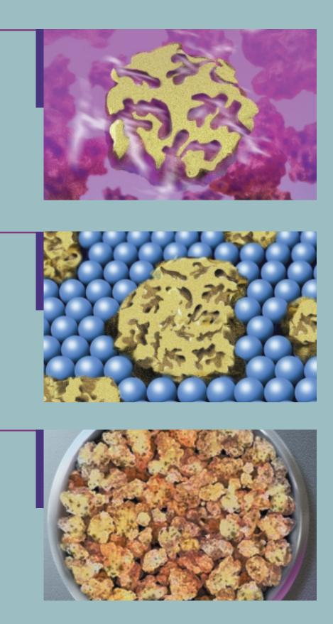
True density - The mass of a particle divided by its volume, excluding open and closed pores.Envelope volume - The external volume of a particle, powder, or monolith such as would be obtained by tightly shrinking a film to contain it.
