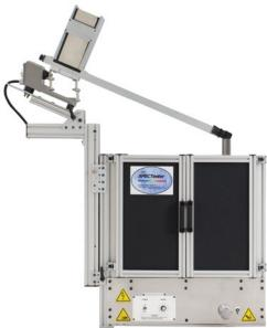
Simulates conditions that cause segregation by particle size, sifting, fluidization, angle of repose, and air entrainment
