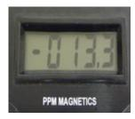
With the sample tube removed, adjust Reading on the display to the positive value of the reading taken with the sample tube filled with the clean mixture of water and oil.
