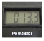
• Fill the tube with a representative sample of the used coolant from the machines, then insert the sample tube into the sample coil and take
