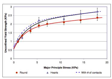
Figure 9: Correction factor applied to round particle strength to correct for the number of contacts per adjacent particle for heart shaped particles
