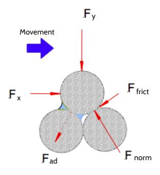
Figure 4: Typical forces acting on a particle in shear
