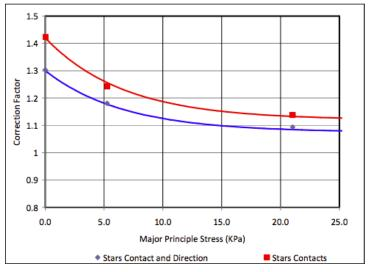
Figure 8: Number of contacts as a function of stress at 16% strain for star shaped particles
