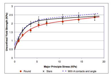
Figure 12: Correction factor applied to round particle strength to correct for the number of contacts and the direction of the contact per adjacent particle for star shaped particles
