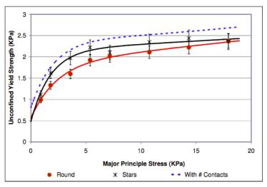
Figure 11: Correction factor applied to round particle strength to correct for the number of contacts per adjacent particle for star shaped particles
