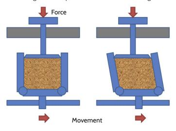
Figure 5: Pure Shear Box (front view)
