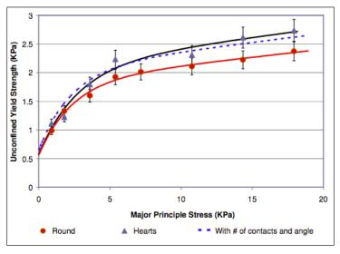
Figure 10: Correction factor applied to round particle strength to correct for the number of contacts and the direction of the contact per adjacent particle for heart shaped particles
