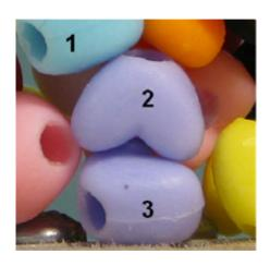
Figure 3: Typical particle contacts between adjacent particles
