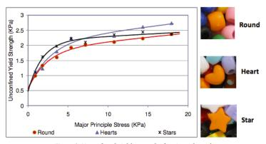
Figure 2: Unconfined yield strength of various shaped particles as a function of consolidation pressure.
