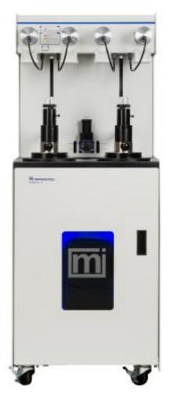
The <u>AutoPore V Series</u> uses mercury intrusion and extrusion to determine total pore volume, pore size distribution, percent porosity, density, compaction/compression, and fluid transport properties.
