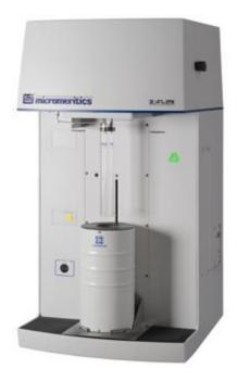
Micromeritics' <u>3Flex Surface Characterization Analyzer</u> is a fully automated, three-station instrument capable of high-throughput surface area, mesopore, and micropore analyses.
