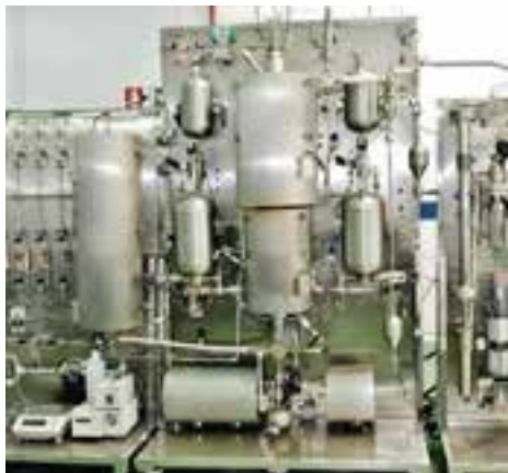
High Pressure Co-Gasification with recirculation
