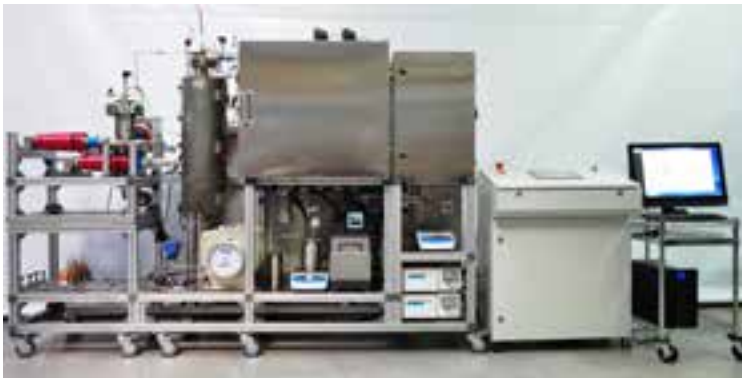
Multipurpose Hydroprocessing Pilot Plant with Solid Feeding at High Pressure
