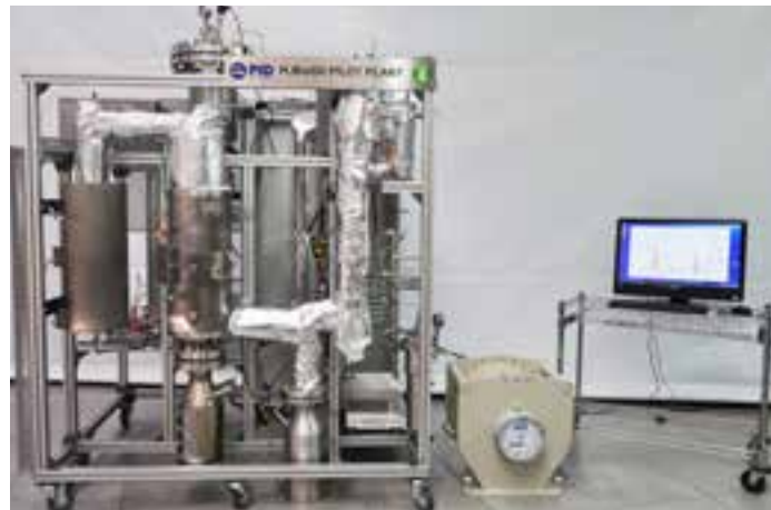
Entrained Flow Pyrolysis of Biomass at High Pressure
