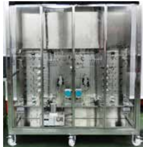
Multipurpose fixed bed reactors pilot plant with transparent enclosure
