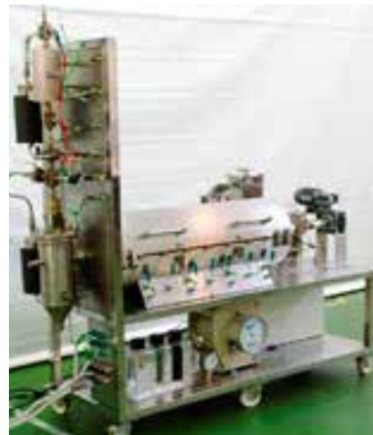
Horizontal Reactor for Slow Pyrolysis
