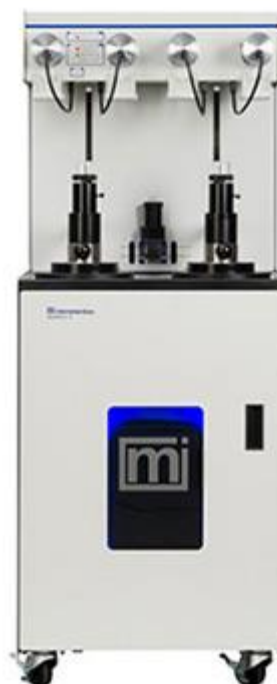
AutoPore V Mercury Intrusion Porosimetry Learn More
