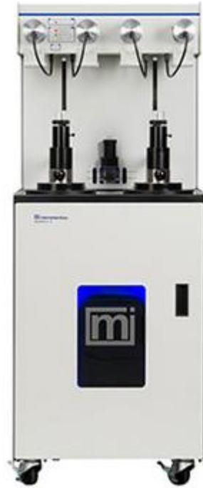
AutoPore V Mercury Intrusion Porosimetry Learn More
