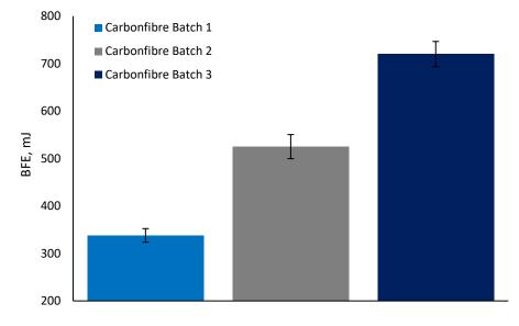
Three samples of carbon fibre strands with an extreme aspect ratio (around 250:1, strand length around 25mm) were tested with the Dynamic Flow methodology, employing a 62mm internal bore vessel in combination with a 23.5mm Blade. The Test Cycle was further modified to incorporate a shallow helix angle and reduced height range to minimise compaction of the strands against the base of the vessel.
