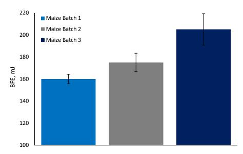
Three samples of maize kernels with average particle size between 8mm and 11mm were tested using the Dynamic Flow methodology, employing a 62mm internal bore vessel in combination with a 23.5mm Blade, to provide over 19mm of clearance between the blade and the vessel wall to prevent particle trapping.
