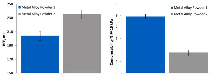
Dynamic Flow and Bulk tests using the FT4 produced statistically significant differences between the two powders. Powder 1 has a lower Basic Flowability Energy (BFE) and higher Compressibility than Powder 2, suggesting that Powder 1 is likely to exhibit more cohesive behaviour manner in lower stress, dynamic processes such as pouring and dispensing.
