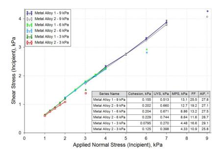
At the three different levels of Pre-Shear stress, the Yield Loci revealed negligible differences between the materials, suggesting that both would exhibit similar behaviour in terms of flow from large hoppers. However, minor variations in the attitude of the best-fit lines applied during Mohr's circle analysis caused significant differences in the values generated for Cohesion and UYS at each Pre-Shear stress, resulting in large differences in the Flow Function values.
