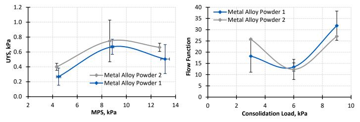
Furthermore, when the variation from repeat tests is considered, the differentiation becomes considerably less robust. The error values in the derived parameters mean that a statistically significant difference is not observed. The right-hand graph also confirms that Flow Function is dependent on consolidating load, and therefore cannot be used as a universal property to describe a powder's flowability.
