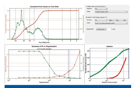
This advanced NLDFT method allows users to determine the pore size distribution of their sample using two isotherms. In this example CO2 adsorption (red) at 273 K and nitrogen adsorption (green) at 77 K are used to calculate a single pore size distribution. Users do not have to cut and paste distributions from CO2 and nitrogen - a single distribution is determined using both isotherms.
