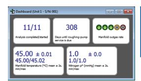
With a single click the TriStar II Plus provides a powerful suite of information that allows the user to maintain the instrument in peak operating condition with real-time analysis views.
