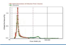
Overlay of BJH desorption and mercury intrusion log differential pore size distributions for alumina pellets
