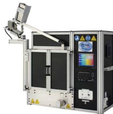
Figure 4. SPECTester used in Segregation Analysis
