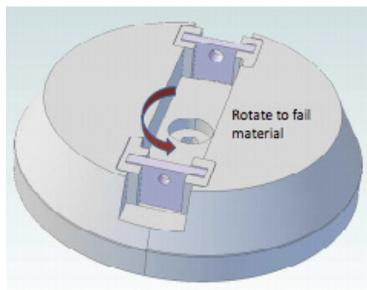
material leaves the cell are used to compute the force needed to fail the compacted material in the conical arch. This data is then used to compute the bulk unconfined yield strength.
