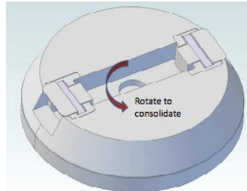
**Step 4:** The fourth step involves stopping the rotation and removing the guards. The bulk material presumably has strength and will arch over the conical cavity. The rotation speed is increased incrementally until the compacted material exits the conical cavity due to centrifugal force. The weight of the material, the position relative to the axis of rotation, and the rotation speed at the point when the
