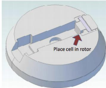
**Step 3:** The third step involves rotating the cell and rotor to a prescribed speed and holding at that prescribed speed for an allotted time. This causes centrifugal forces to act on the bulk material in the conical cell and compact the material within the cell. The rotor speed and the weight of the material, along with the position relative to the axis of rotation, are used to compute the consolidation pressure.
