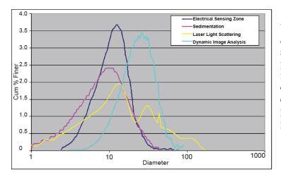
Wollastonite particles are rod-shaped. Since the apparent dimensions of a rodshaped particle can vary drastically depending on its orientation, the detection methods that were affected by particle orientation (laser light scattering and dynamic image analysis) exhibited larger particle size measurements and broader peaks.
