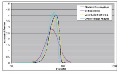
Glass spheres, as expected, produced the most consistent results for the different techniques. Since the particles are spherical, their orientation has no effect on their measurement. Microscopy of the sample indicated that the glass spheres contained air bubbles in variable sizes, reducing somewhat the density of some of the spheres. Because of this, the SediGraph detects some of the particles as being undersized and, therefore, widens the distribution and shifts it to a slightly finer size.
