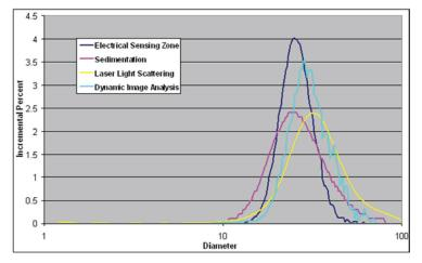
Garnet crystals approximate cubic shapes. Since the diagonal of a cube is approximately 30% longer than a sphere of the same volume, larger particle size is reported by methods that take orientation into account (laser light scattering and dynamic image analysis).
