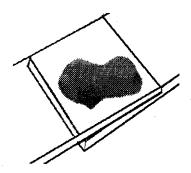
Take another clean slide and place it on top of the first slide overlapping only half way, pressing the honey-sample mixture between the two slides. Separate the two slides; this shears the particles. Place the slides back together, again overlapping by half and then separate them again. Repeat this procedure several times.
